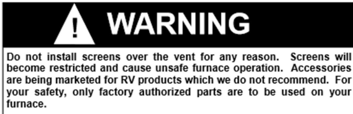
Exterior vents must be free from obstructions and properly vented to the atmosphere for best performance and health purposes. Inspect the following:
