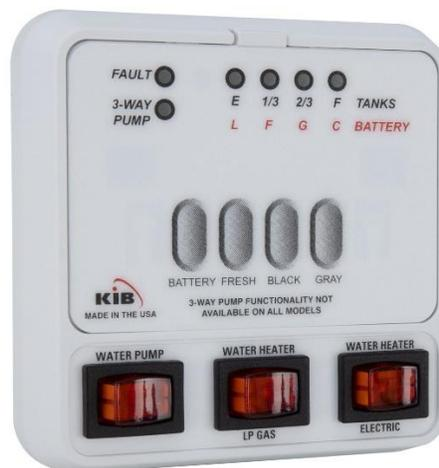
The switch on the lower left corner is for the water pump operation. When in the “ON” position, the pump will run until 40 - 45 PSI is achieved. The pump will shut off and restart at 20 pounds of pressure. Turn pump switch “OFF” when pump is not in use.
